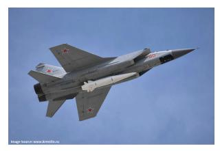
Figure 4: Russian Kinzhal medium-range ALBM on Mig-31 Interceptor. (Capable of maneuvering aerodynamically after boost.)
