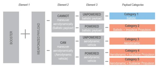
Figure 5: Combinations of fundamental missile system elements.
