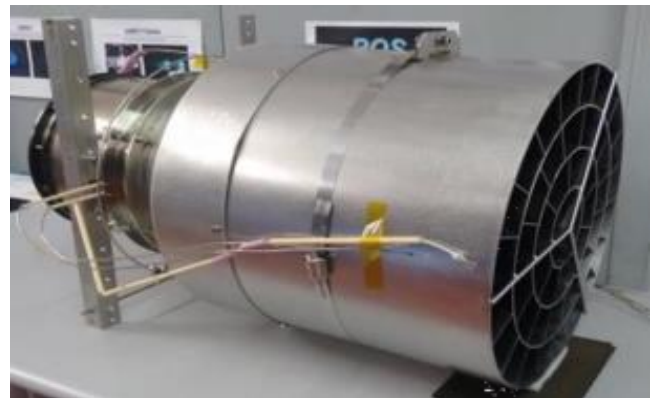
Figure 4: Air scoop design integrated with a Hall thruster. Investigated by Barral and Walpot and ground tested by Sitael. The honeycomb structure is designed to capture more air particles by minimizing the backflow to increase pressure and density at the end of the air intake. Sources: S. Barral, L. Walpot, “Conceptual Design of an Air-Breathing Electric Propulsion System,” IEPC-2015-271, 2015. T. Andreussi et al., “Development and experimental validation of a hall effect thruster ram-ep concept,” International Space Propulsion Conference, SP2018-00431, 2018.
