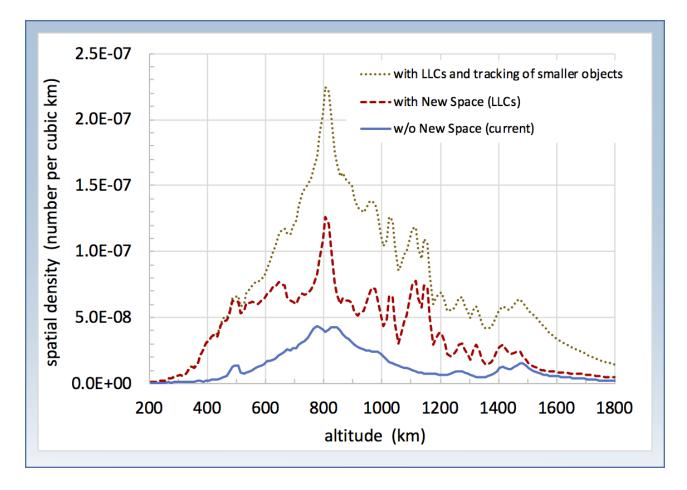
Figure 3: Spatial density of objects in LEO with and without New Space activity. Adding New Space LLCs will increase the density at all altitudes due to replenishment, disposal, and failed satellites. Adding the smaller objects that would appear with an improved tracking system could increase the density at all altitudes even more.
