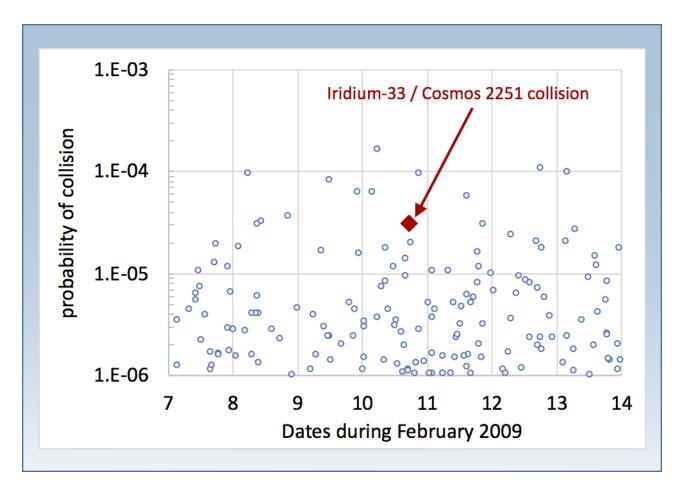
Figure 2: Iridium constellation conjunction probabilities during week of Feb 7, 2009. Under current tracking accuracies, the actual collision between Iridium-33 and Cosmos 2251 did not stand out from other conjunctions that week as being noticeably dangerous.
