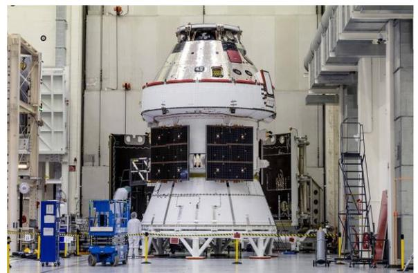
**Figure 2: Orion crew vehicle with solar panels attached.**
